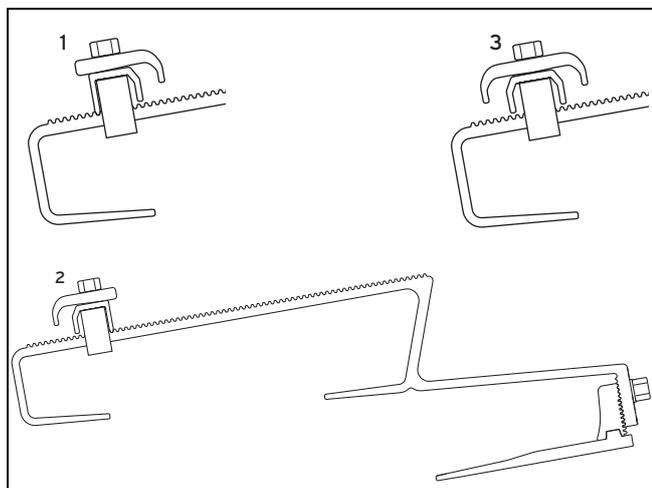
1 Unterer Dachanker                      3 Mittlerer Dachanker
